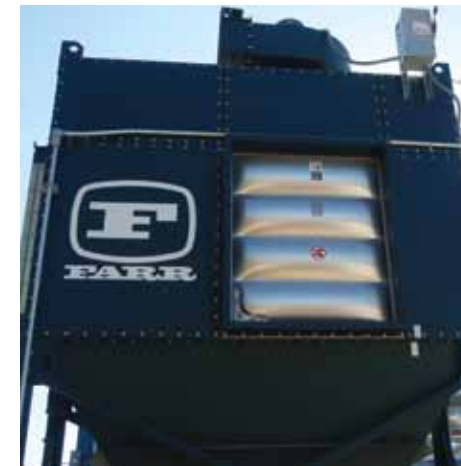
Explosion Vent-ATEX approved and NFPA compliant rupture panel.
